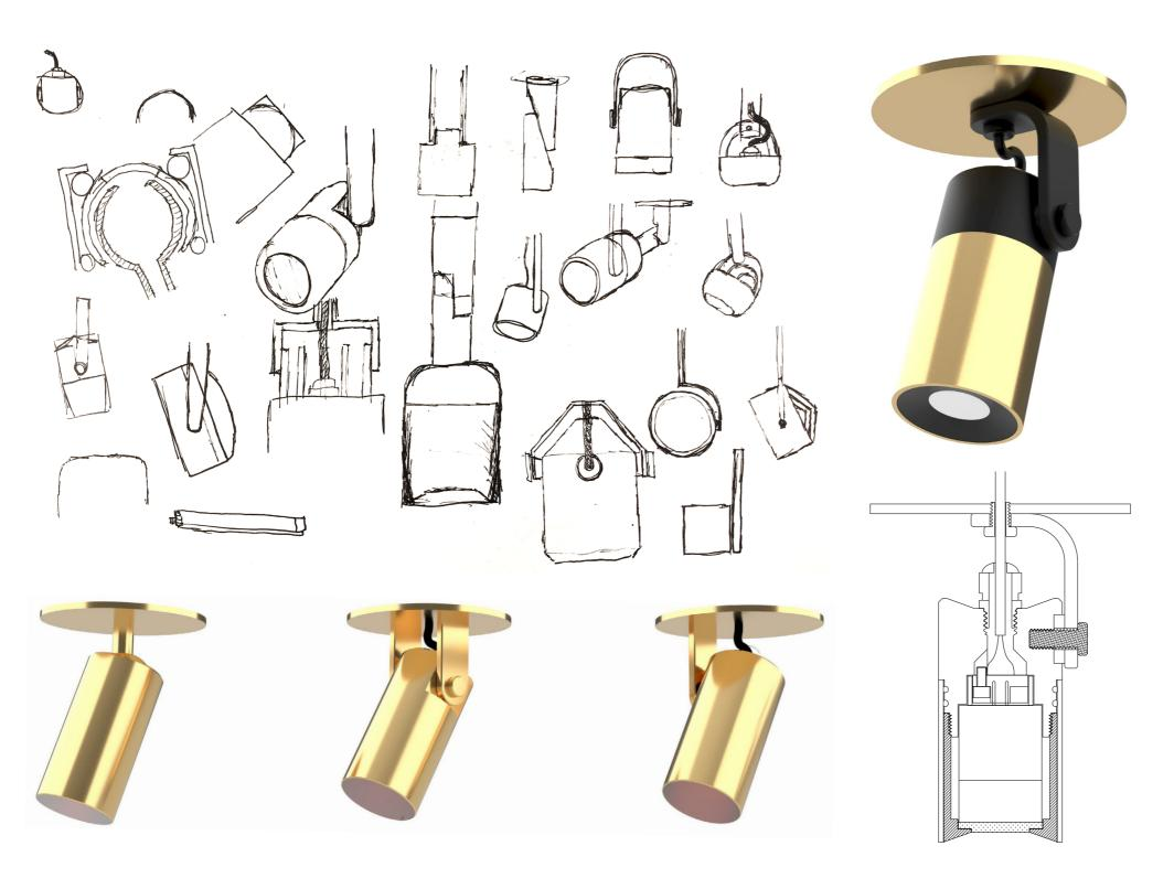
Tim was contracted to Alma Lighting to produce an economical spot light design for the 38 Series which utilises the variety of metal types which are available in the same \$\phi 38mm\$ size tube. Because of this design, the light can be customized to have stainless steel, brass and copper finishes, as well as any range of powdercoat colours.
